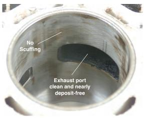
Following 534 hours in service, the cylinder bores demonstrated 0.00% scuffing and the cross-hatch pattern is 100% intact. The exhaust ports are nearly deposit-free. Results prove the superior protection and clean-burning properties of HP Marine.
